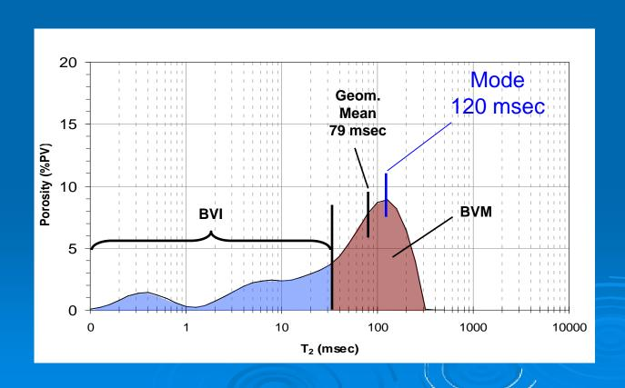
*Notes by Presenter*: A T2 spectrum from a sandstone has a general form like this. The commonly measured variables are BVI, BVM, and the Geometric mean. Note that the mode is a much better indicator of the dominant pore size than the geometric mean. Variables are derived from the entire T2 distribution, and it is assumed that the entire distribution is determined.
