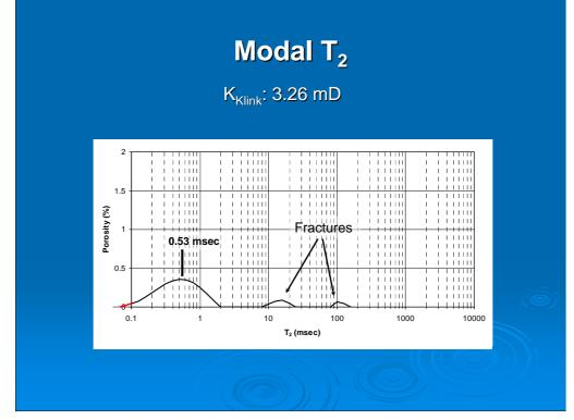
**Notes by Presenter:** Representative spectra from sample of tight gas sand with fractures. Should we lump these fractures with BVM? Note that the mode is approximately 0.55msec, and at this point the 'good' part of the spectrum is incomplete and is missing a tail....(How do we get BVI from this?).
