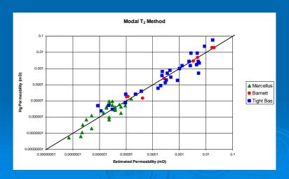
**Notes by Presenter:** Finally, let's look at the results obtained using the Modal T2 time. Using MICP data to seed the regression, we can derive the parameters for each rock type and obtain results that have very little deviation from the measured values. Note that the small amount of deviation that is present is symmetrically distributed around the 1:1 line.
