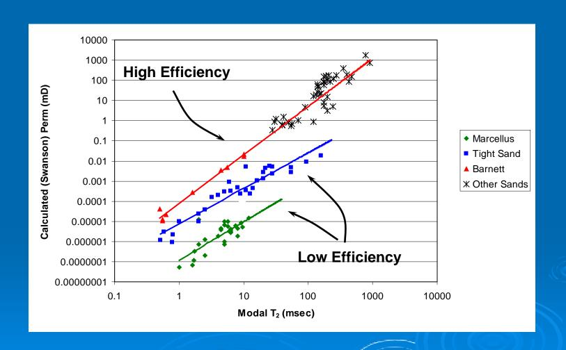
*Notes by Presenter*: If we compare the Barnett with reservoir sands, we see that, in terms of pore size and permeability, the Barnett shale has a pore network that is just as efficient as that of many reservoir sandstones. This suggests that the dry-gas generation phase creates enough pressure either to re-open pathways that were closed during compaction, or to generate microfractures which substitute for these pathways.
