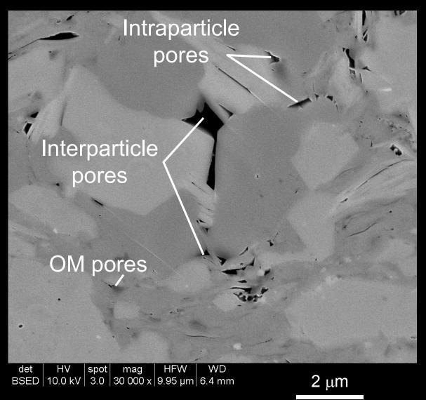
Interparticle pores between grains with overgrowths
