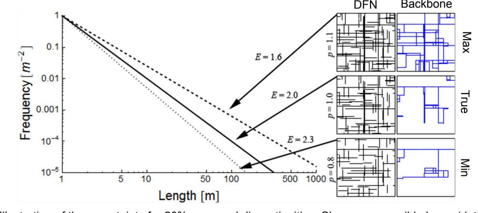
Figure 5. Illustration of the uncertainty for 20% censored discontinuities. Shown are possible lower (dotted line, bottom DFN), true (solid line, middle DFN) and upper (dashed line, top DFN) estimates for the power-law exponent E and the density p.
