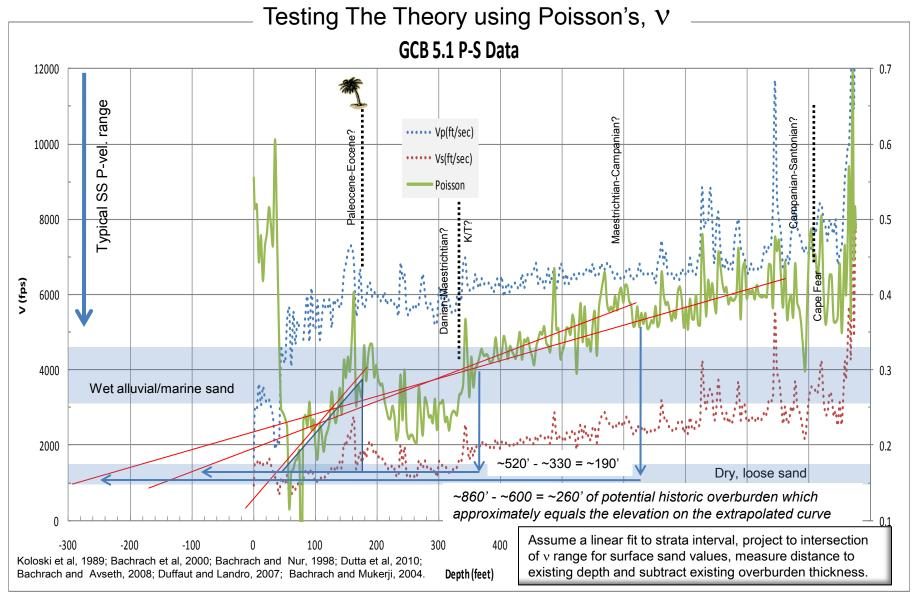
If using the assumption that deposition proceeds to least compressive energy (zero overburden), and using typical P-S and v values for unconsolidated surficial sands, and extrapolating a "normal" increasing-with-depth acoustic signature to its ultimate unconsolidated value, and allowing for current burial status, then historic overburden thickness might be derived.
