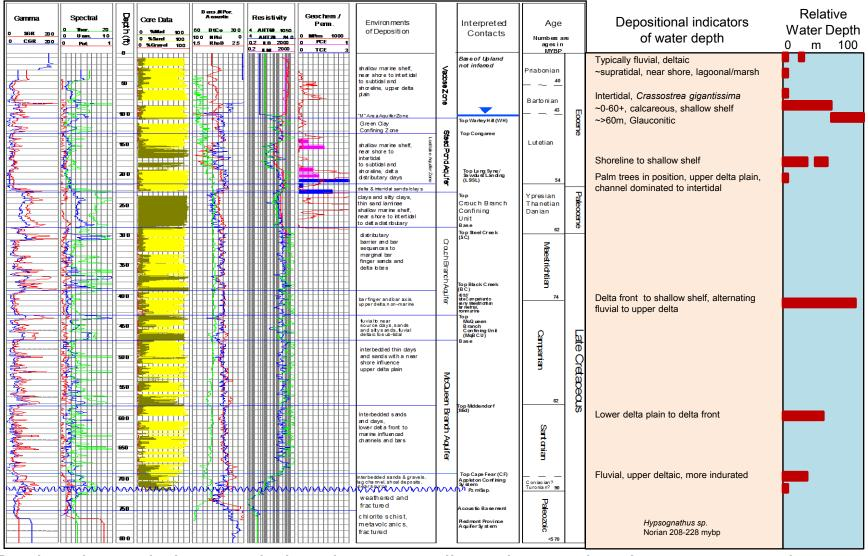
Regional correlations and abundant core allowed us to develop a very good stratigraphy and depositional history tied to locally interpretable geophysical signatures. Using LandMark it was possible to visualize multiple logs, core and seismic data in one view to develop Chrono-, Litho-, and Hydro-stratigraphy.
