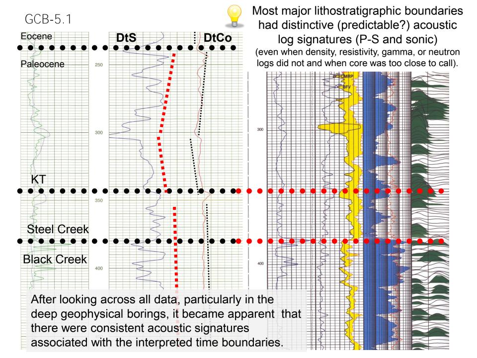
Comparison of Chronostratigraphic, Lithostratigraphic and Hydrostratigraphic Units with approximate seismic response. The sonic data typically had predictable signatures associated with all known major unconformities.
