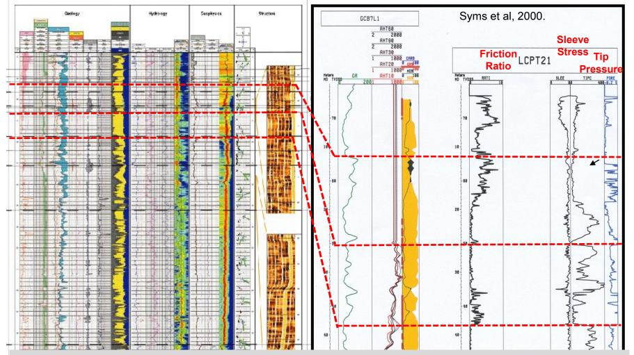
Advanced Geophysical Log to Standard Geophysical Log to CPT and Core.
