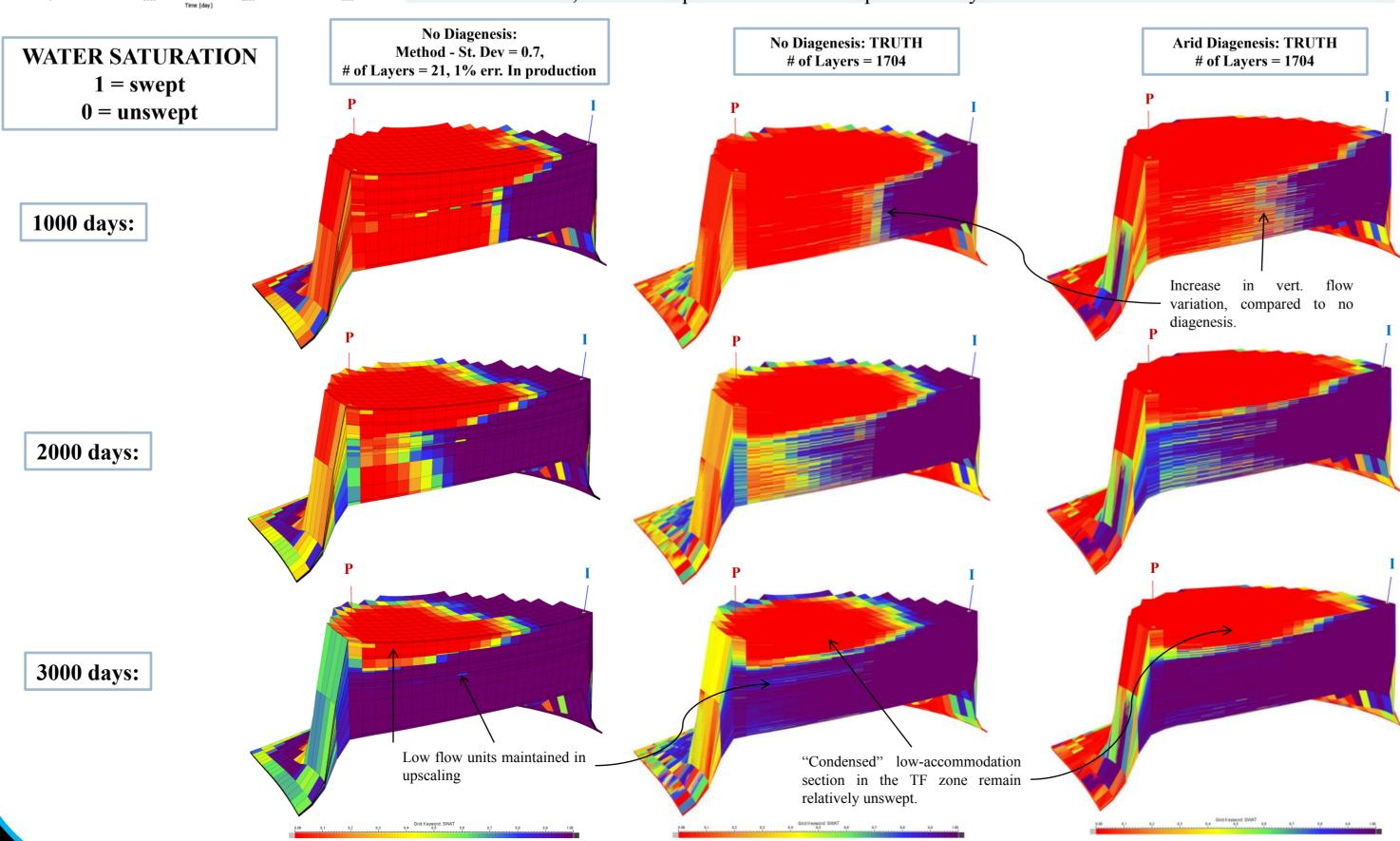
Diagenesis, Arid and Humid "Truth" simulations. Volumes produced are ormalised against the volume produced from the "truth" model
