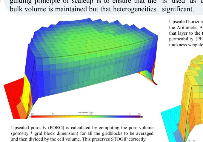
Upscaled horizontal permeability (PERMX and PERMY) is calculated by the Arithmetic Average, weighted by the thickness of each gridblock in that layer to the total thickness of all layers to be amalgamated. Vertical permeability (PERMZ) is taken as the Harmonic Average, but is also
