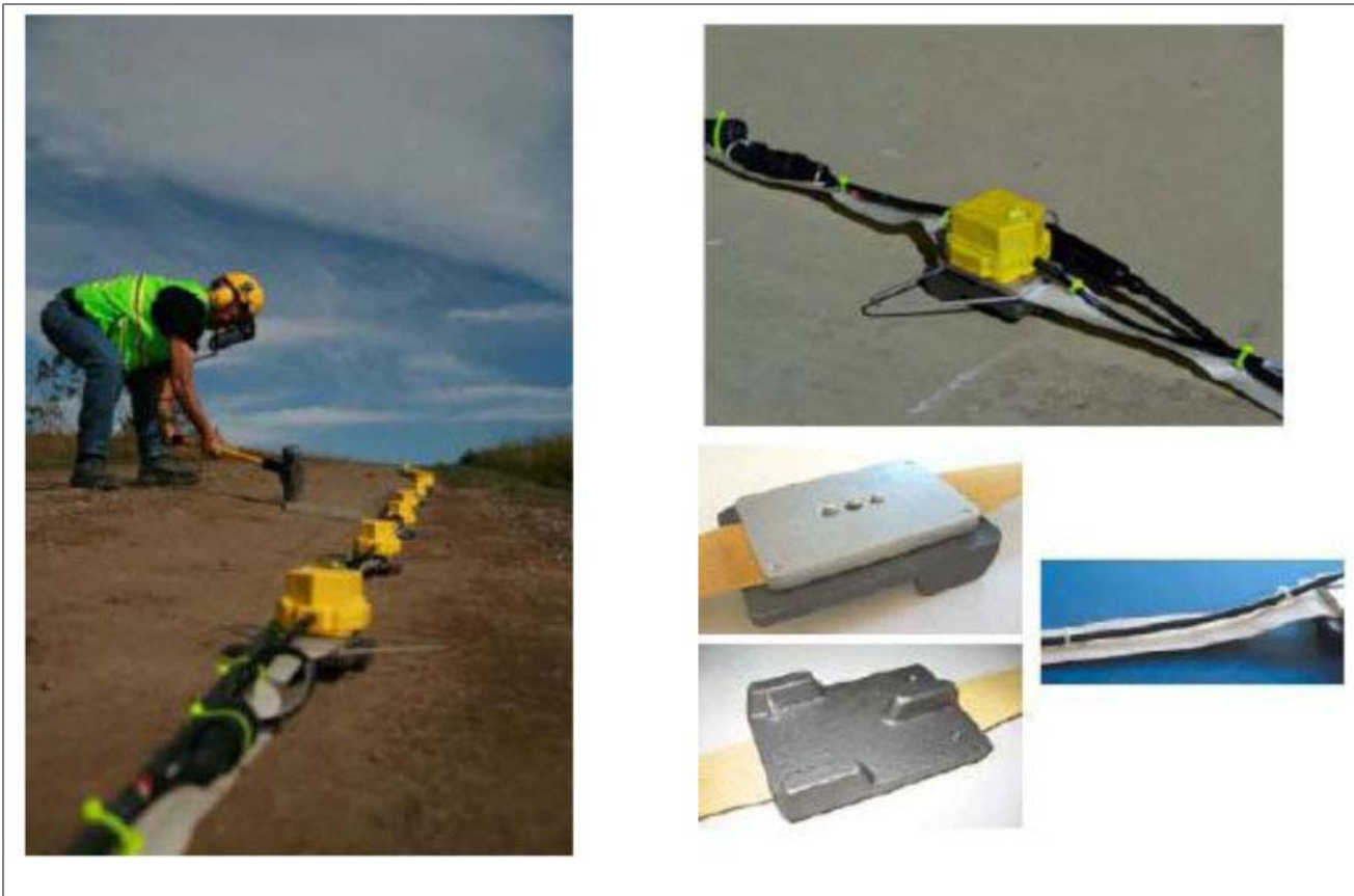
Figure 3. Land streamer in SSR survey.
