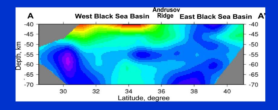
Distribution of P-wave velocity with depth in the western (WBS) and eastern (EBS) parts of the
