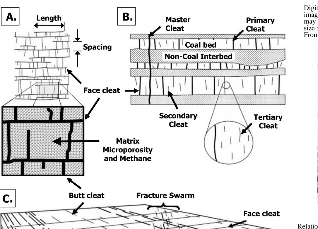
Digital images of the cleat system. The images show irregularities in the cleats that may remain open and connected despite cleat size reduction in higher stress environments From Karacan and Okandan.<sup>57</sup>
