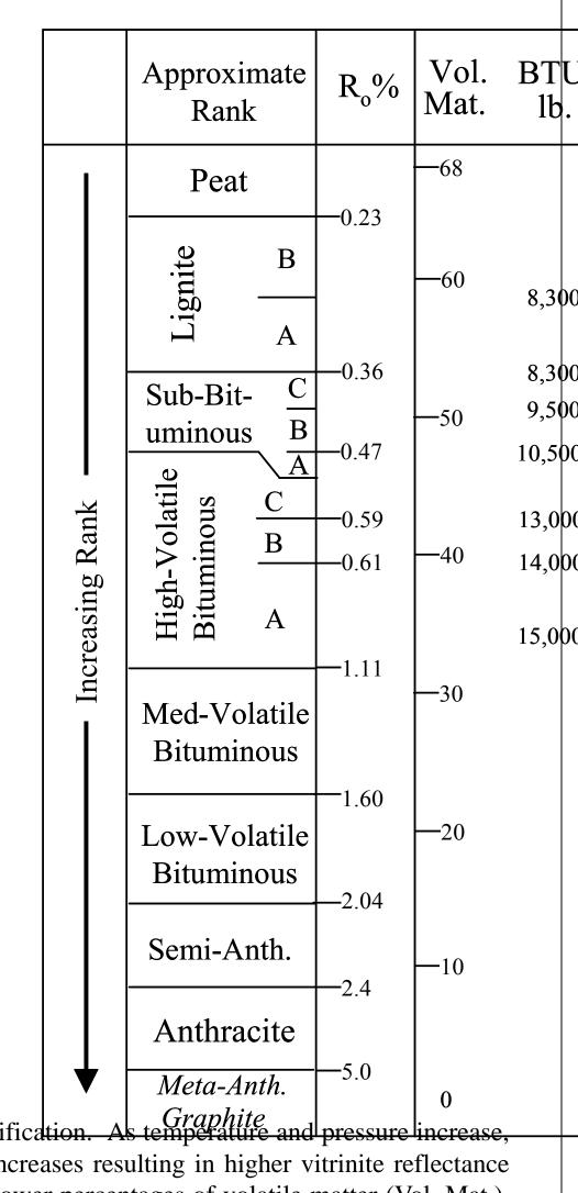
Coal rank classification. As temperature and pressure increase, the coal rank increases resulting in higher vitrinite reflectance values (R<sub>o</sub>%), lower percentages of volatile matter (Vol. Mat.), and higher heating capacities (BTU/lb.). Adapted from Stach et al.<sup>53</sup> found in Mukhopadhyay and Hatcher.<sup>54</sup>
