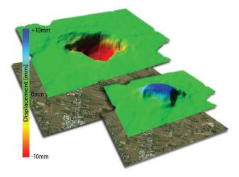
Above: two images taken from an animation showing the evolution of vertical displacement as gas is injected and extracted from the gas storage reservoir
