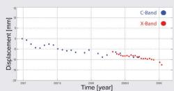
■ The new X-band satellites have a significantly higher temporal sampling rate than C-band. Revisiting times can be as low as 4 days, compared to 24 or 35 days with C-band, leading to more effective monitoring of reservoirs.
