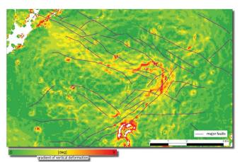
*Above:* gradient field of cumulative vertical deformation. Red areas indicate rapid changes in surface deformation velocity and are likely to correspond to active faults / fractures in the overburden.
