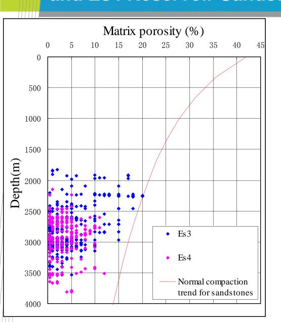
The matrix porosities were estimated from thin-sections. The sandstones do not have anomalously high porosities.
