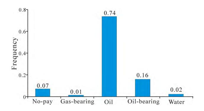
The overpressured reservoirs are dominated by either oil saturated (74%) or oil-bearing (16%) reservoirs.
