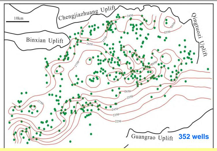
The top of the overpressure zone ranges in depths from 2200 m to 3000 m closely mimicking the depths of the source rocks.
