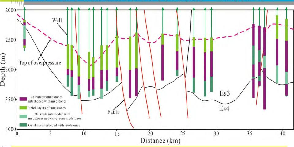
The top of the overpressure zone is associated with thick layers of mudstones/calcareous mudstones. Internal fractures and vertical faults are present in Es3 and Es4.
