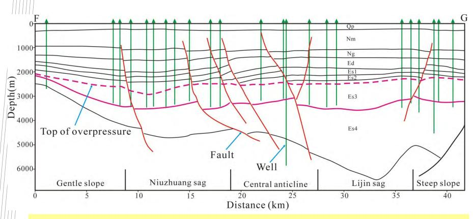
The top of the overpressure zone ranges from 2200 m to 3000 m and increases with the burial depths of the source rocks. The temperatures for the top of overpressure zone are *ca* 87-123°C corresponding to estimated vitrinite reflectance (Ro) of 0.5-0.75%.
