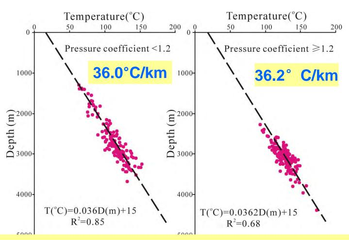
The similar geothermal gradients suggest that the overpressured sandstones do not have anomalously high porosities as compared with the normally pressured sandstones
