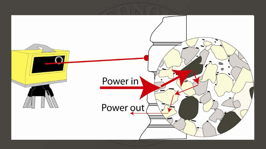
Intensity is the ratio of the power of reflected light to power of emitted light.
