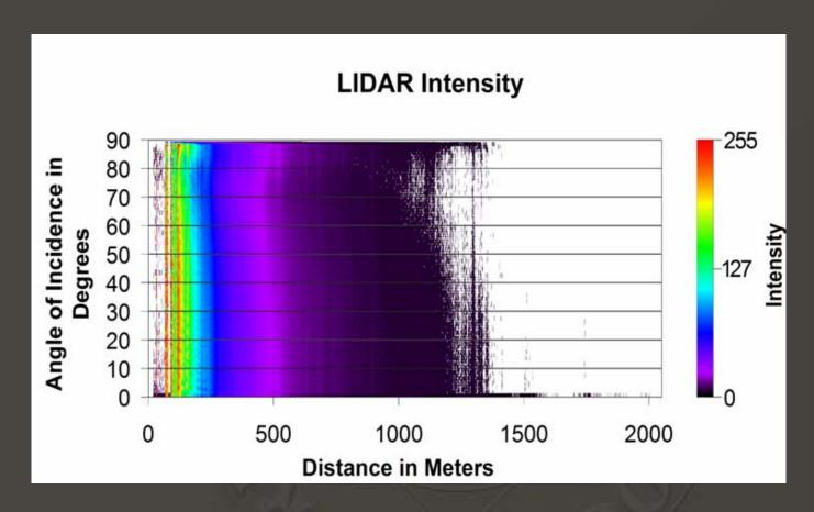
Distance has the biggest impact on intensity and correction can be made for it.
