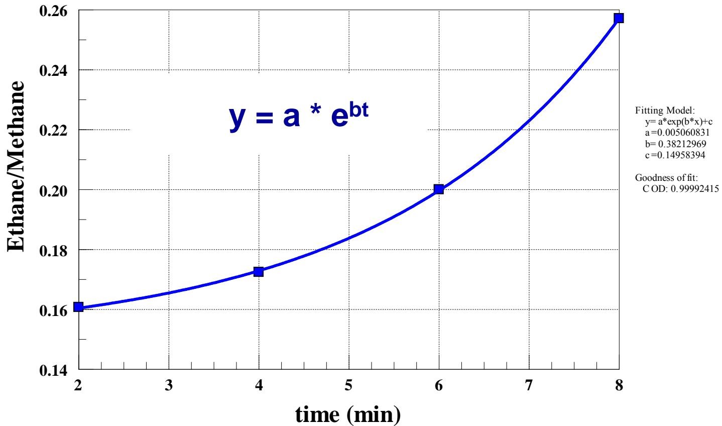
Charge 500 psi, degassing under vacuum, ambient temperature
