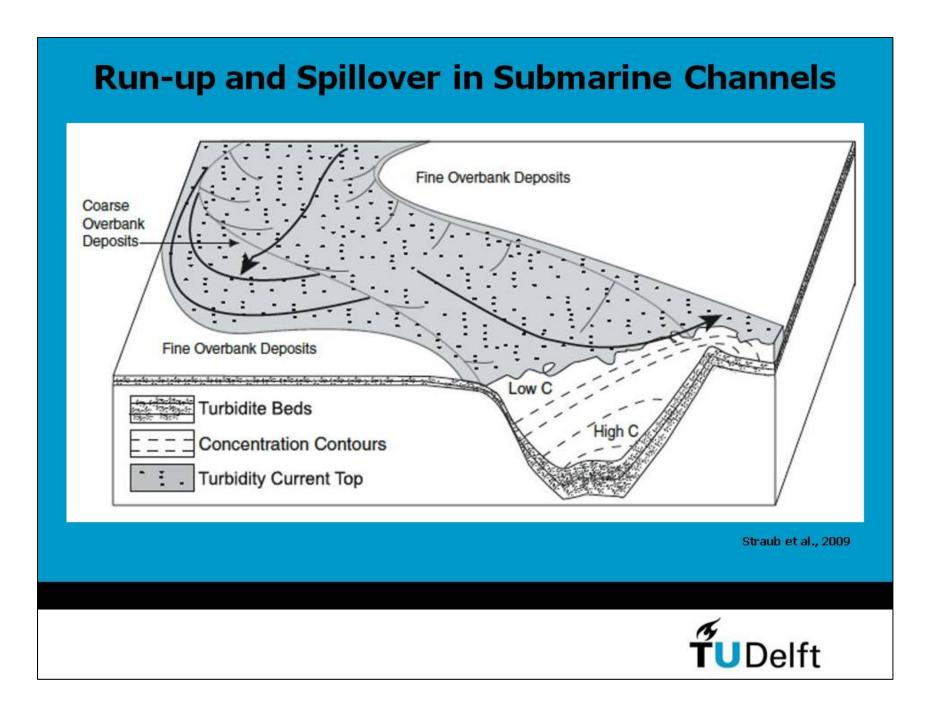
This is an experimental result, although I don't know how widely applicable their coarse-grained deposits on the outer bank are.
