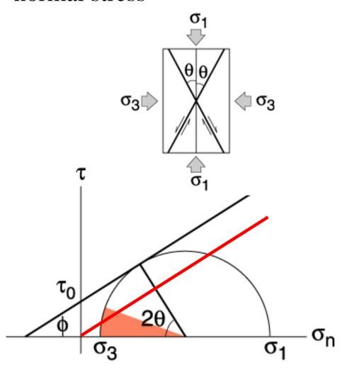
2. Hydraulic opening translating to shear along intersecting fractures
