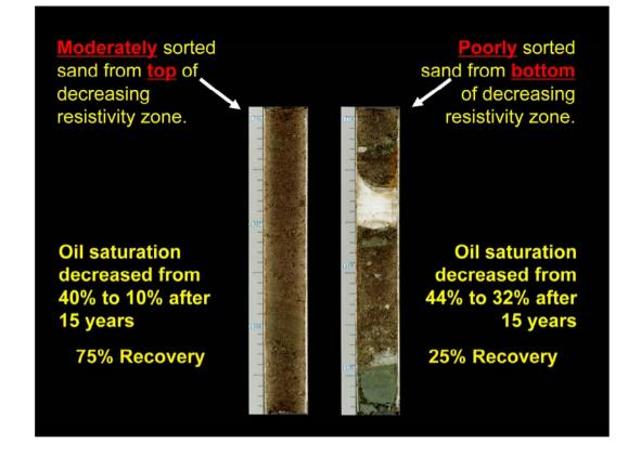
On the left is a moderately sorted sand from the top of a decreasing resistivity zone, and on the right is a poorly sorted gravel from the bottom of the same zone. After 15 years of steam injection, oil saturation at the top of the zone decreased form 40% to 10% for a rather respectable 75% recovery rate. However, over the same time period, oil saturation at the bottom of the zone decreased from 44% to 32% for only a 25% recovery rate.
