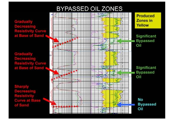
Here is a log with resistivity on the left and oil saturation on the right. Produced sands are shown in yellow. At the bases of the upper two sands there are significant zones of bypassed oil shown in green. The log signatures for both of these sands exhibit gradually decreasing resistivity values across the bypassed-oil intervals. The lower sand's resistivity profile shows a sharp decrease at its base and there is no bypassed oil.
