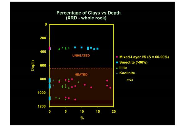
A second suite of samples was collected from decreasing-resistivity zones, some heated and some not heated. These analyses distinguished between smectite and mixed-layer illite/smectite and also characterized the mixed-layer clays. The unheated samples contain relatively pure smectite as might be expected from shallow burial diagenesis in the presence of fresh groundwater. In contrast, the heated samples contain random-ordered mixed-layer illite/smectite containing 60-90% smectite layers.
