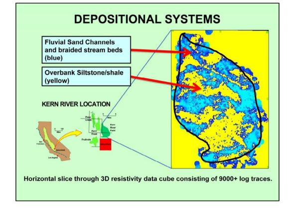
This is a horizontal resistivity slice based on more than 9000 well logs. The distribution of sandstone and conglomerate channels is shown in blue and the more widespread siltstones are shown in yellow.
