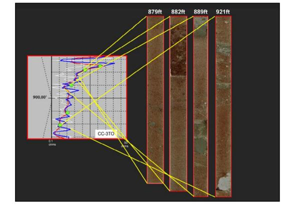
On the left is a typical resistivity log from one of these zones. The cores on the right show the change from moderately sorted sand at the top to poorly sorted gravel toward the base. The green dots show locations of samples collected for analysis.
