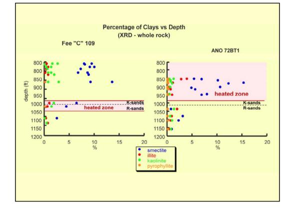
These diagrams show the composition of clay minerals in unheated and heated samples. Illite probably reflects fine-grained micas. Kaolinite is minor and shows a slight reduction due to heating. Smectite shows an increase in both heated zones. These analyses did not characterize smectite type or distinguish smectite from smectite-rich mixed-layer illite/smectite.
