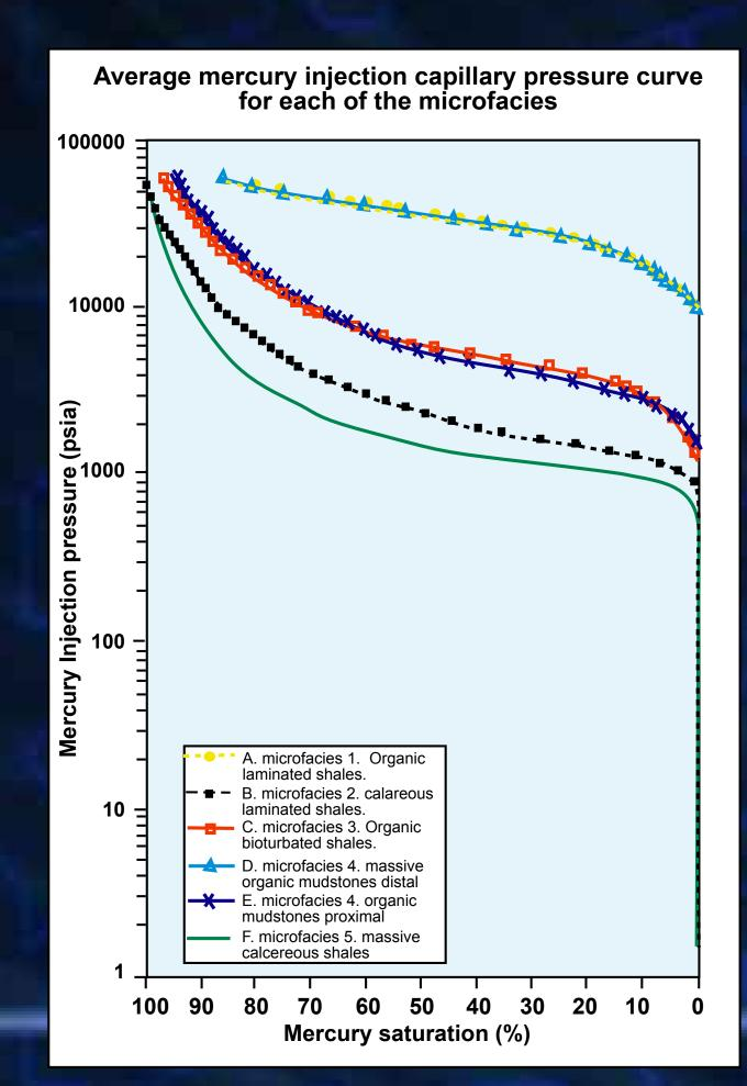
Distal marine (TST) shales (microfacies 1 and 4) exhibit the "best" seal character based on MICP analysis.
