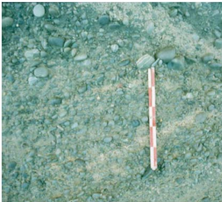
Figure 2. Light coloured mud layers with late Quaternary Burnham Formation gravels, Canterbury Plains. Such layers follow zones of higher permeability (such as foreset stratification), and are introduced into the bed through percolation of fines downward and laterally through the deposit. Scale is 50 cm with 10 cm divisions.
