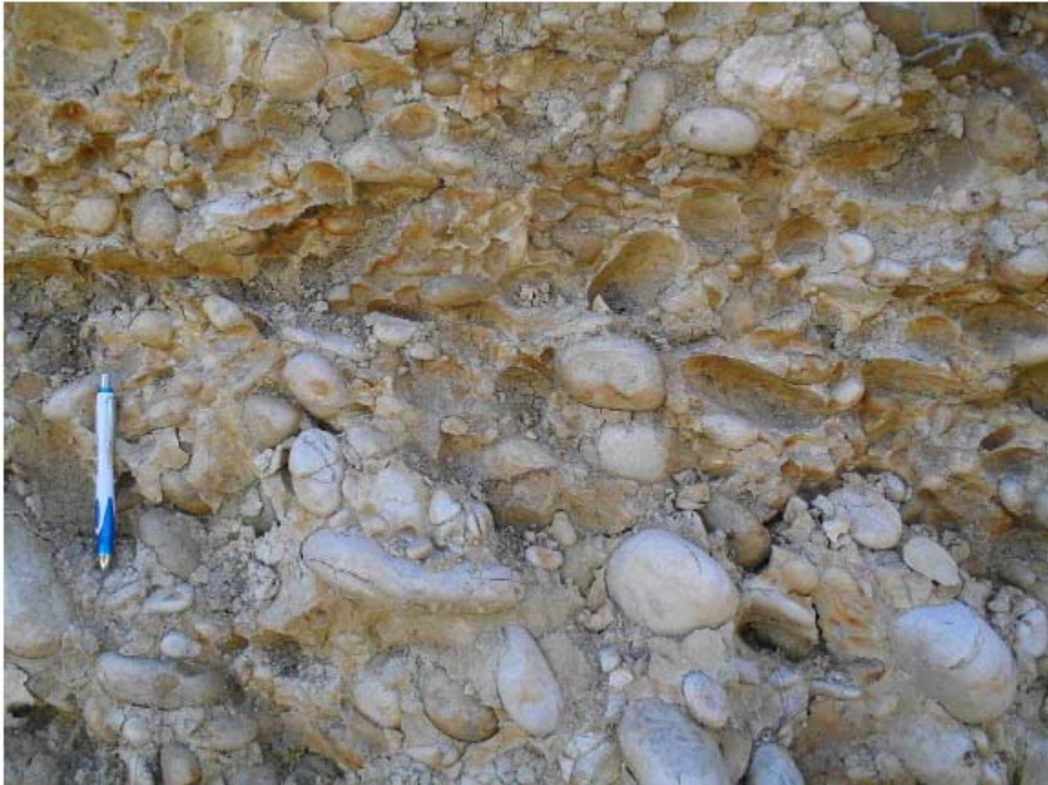
Figure 3. Clay-bound gravels in the Pliocene Moutere Gravels, Nelson. Most of the matrix in this unit is silt introduced after deposition of the fluvial gravel deposit. Pen for scale (left).
