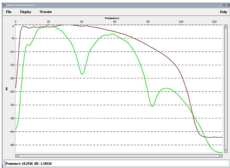
Figure 2: Average amplitude spectrum of a stacked data volume from West of Shetlands, UK. Green and red curves show the spectrum with and without application of the deghosting strategy discussed in this paper, respectively.
