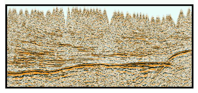
Stack with Simulated Annealing, Monte Carlo-Derived statics
