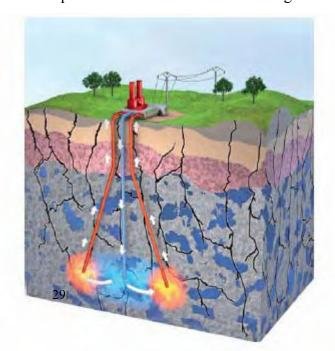
Cooled water is re-injected in the fractured granite by a central injection well (in blue).(after Genter et al., 2009)
