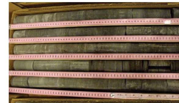
Shale with very few carbonate beds from Well No. 44 (Core 2982) from 164.6-167.5 m.
