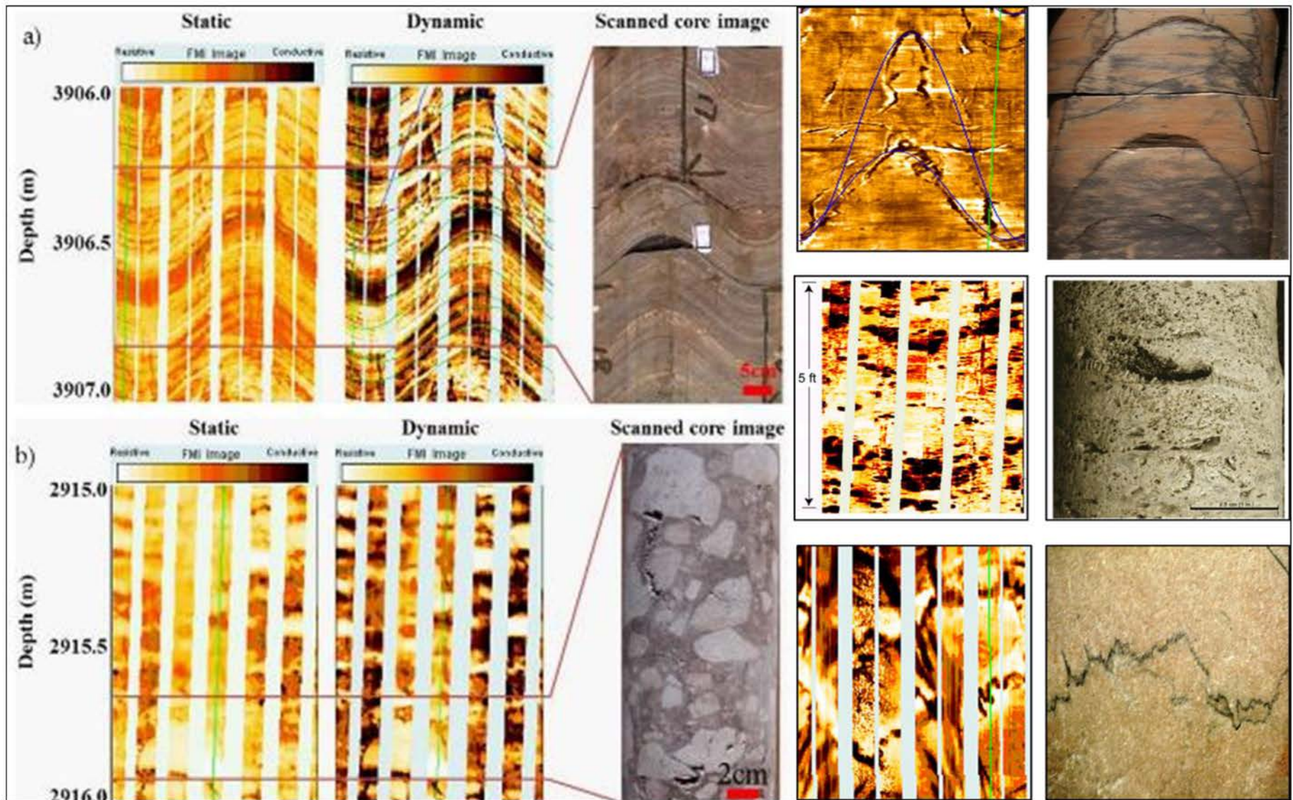
Figure 2. Borehole images showing the core-features, (a) cross-bedded sands, (b) diagenetic nodules, with fractures, vugs, and stylolites in right hand side of the snapshot.
