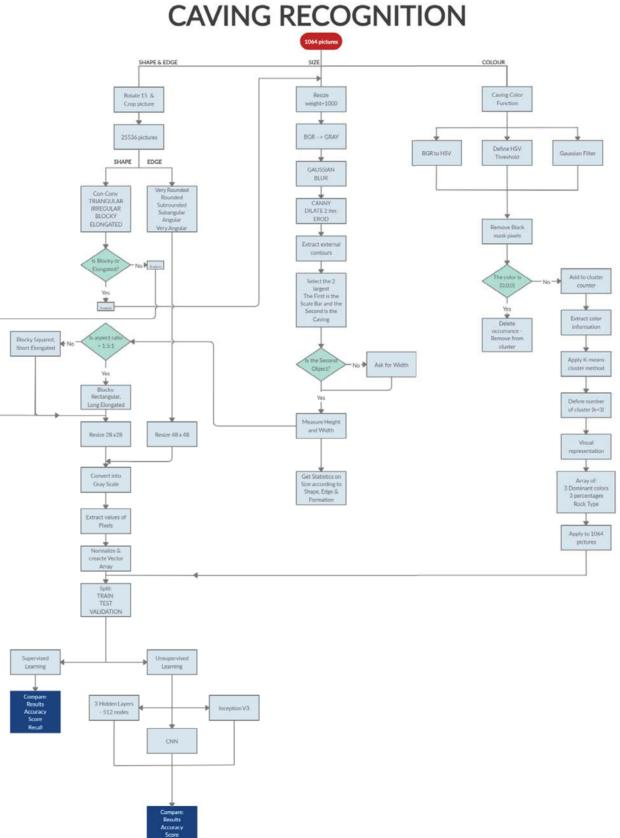
he process of extracting the features of each caving can be summarized in three fronts: Shape & Edge, Size and Colour. The first two are within the interest of the project and the last two are used to help recognize the correct caving
