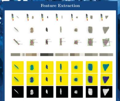
ach picture is cropped within the desired area, resized and turn each pixel into values to ge e following array: 1,064x3,136 (rows x columns). Where each row is a picture and each olumn is a feature with a value between 0-255 as an 8-bit grayscale picture. Feature traction also includes the size of the caving and the most dominant colours using K-means
