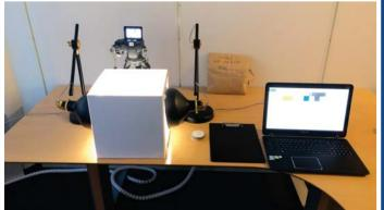
indard dataset was built from scratch using a photobox with consistent light cond rough all the samples. It is important to have a template with the elements needed to antee the position of all the elements in the picture, including the position of the ing and the focus on it.
