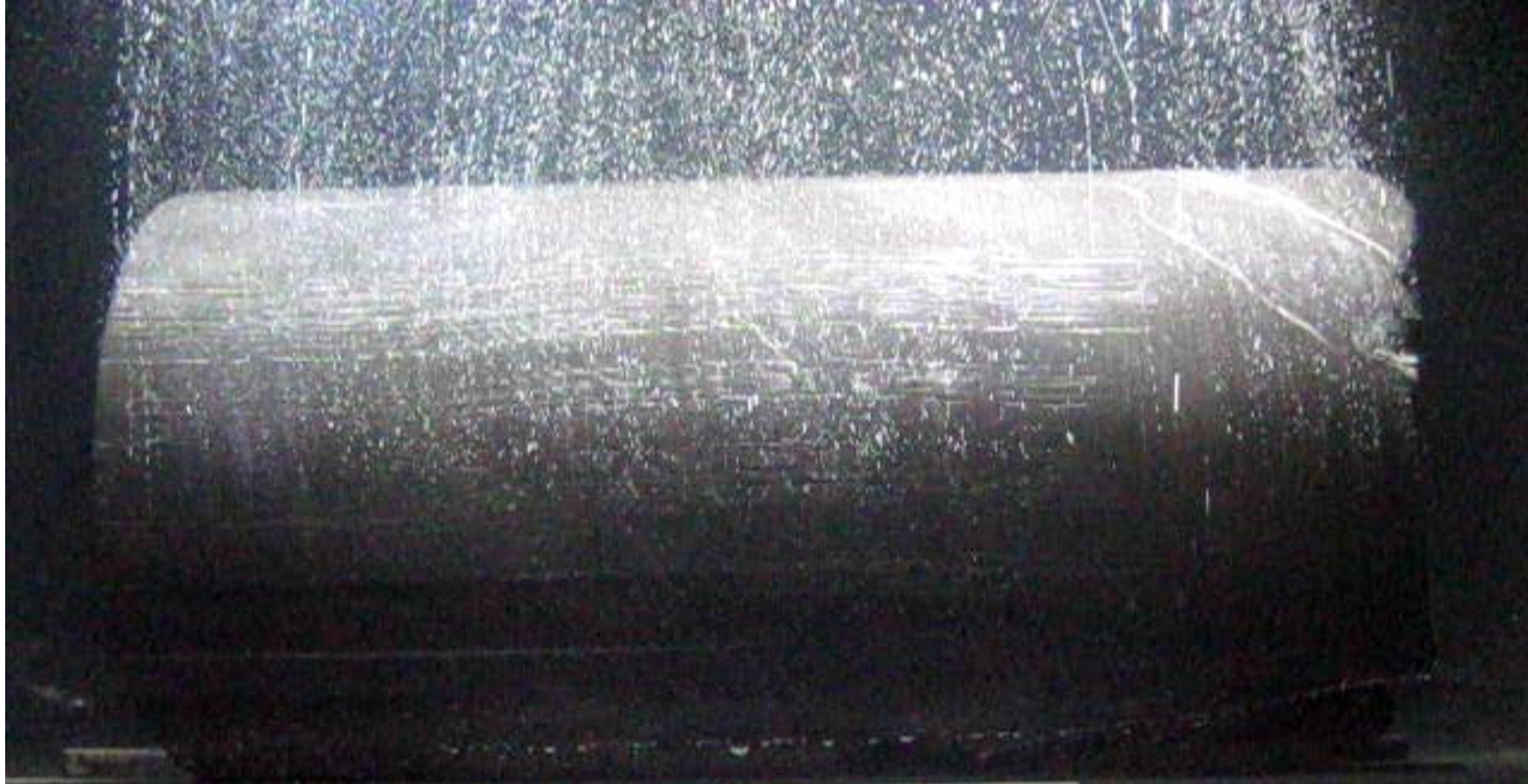
Natural Gas Desorbing from Tight Rock Core (Depth 5,336 ft)
