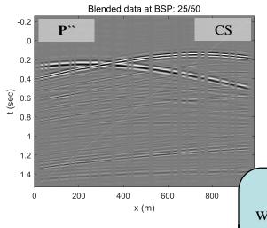
Shot-generatedwavefields interfered, frequency-banded, non-uniformly and under sampled.
