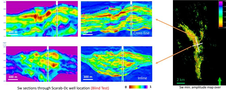
Sw min. amplitude map over Scarab channel 1 reservoir
