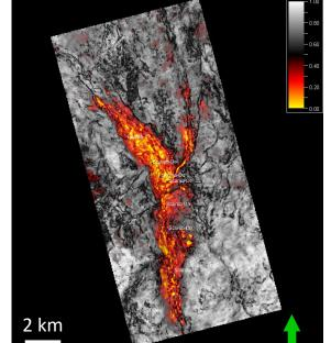
Sw minimum amplitude map overlaying variance map over Scarab channel 1 reservoir
