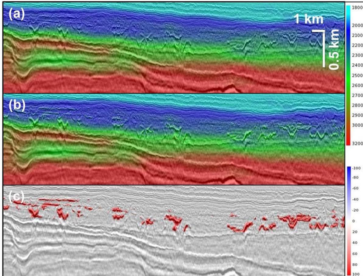
Figure 1. Inline stack section in depth with interval velocity overlay (a) before, and (b) after insertion in injectites. (c) Velocity difference following insertion of 5% speedup relative to background velocity. Note Hilbert transform successfully and accurately isolates the top and base of the injectite bodies enabling suitable insertion of speedup in preparation for following GMO picking and high-resolution tomography.
