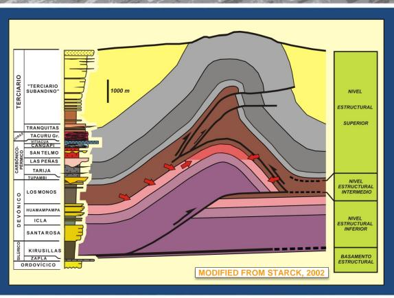
FRACTURED QUARTZITES IN LARGE, DEEP ANTICLINES
