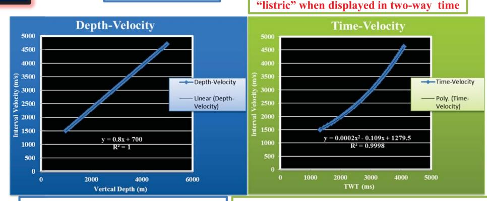
Linear depth-velocity relationship on Synthetic Depth-Interval Velocity Model
