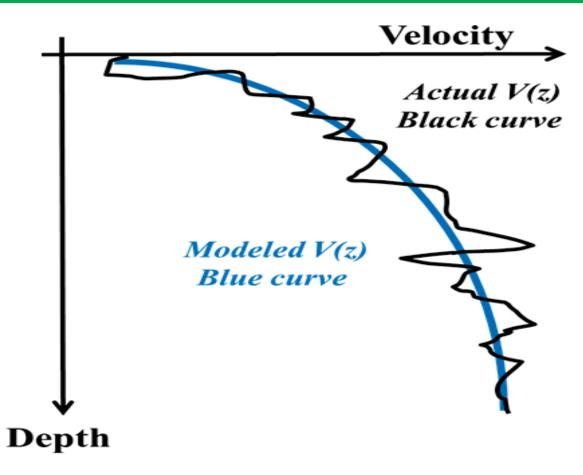
Analytical function describes a smooth variation of velocity with depth, much smoother than the high frequency fluctuations observed on well interval velocities.
