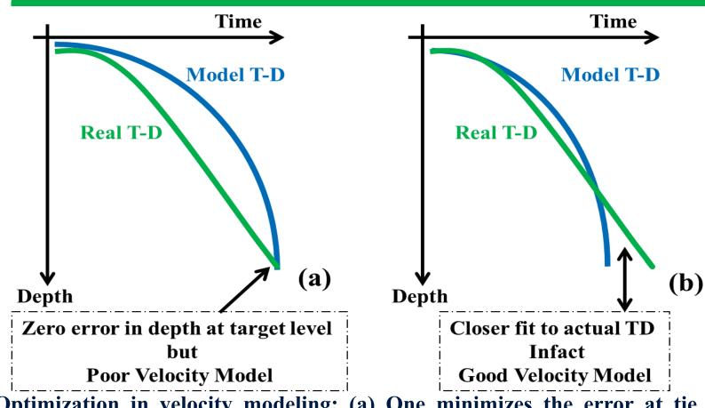
Optimization in velocity modeling: (a) One minimizes the error at tie point (direct conversion) but model does not represent the true geology but (b) when one honors the true function the error at the tie point increases.
