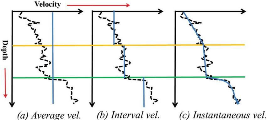
Three levels of detail in modeling velocity. (a) Simplest level is average velocity from top to down (b) Bit more complex is: assign a constant interval velocity to each layer within a given well (c) Complex one is: instantaneous velocity modeling of the dataset; this type of curves provides velocity variation over very small depth increments.
