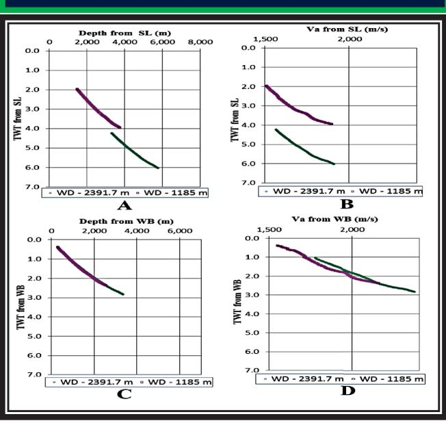
Effect of water column on time-depth and average velocity curves. Variable water depth obscures compaction relationships. (A) time-depth curve with regards to sea level (B) average velocity with regards to sea level (C) time-depth curve with regards to sea floor (WB); (D) average velocity with regards to sea floor. TWT = vertical two-way travel-time; SL = sea level; WB = Water Bottom
