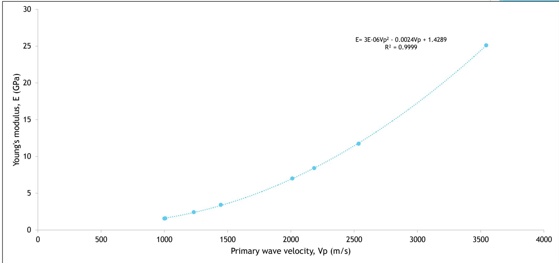
Fig 2: The graph of Young's modulus (GPa) against the primary wave velocity (m/s)
