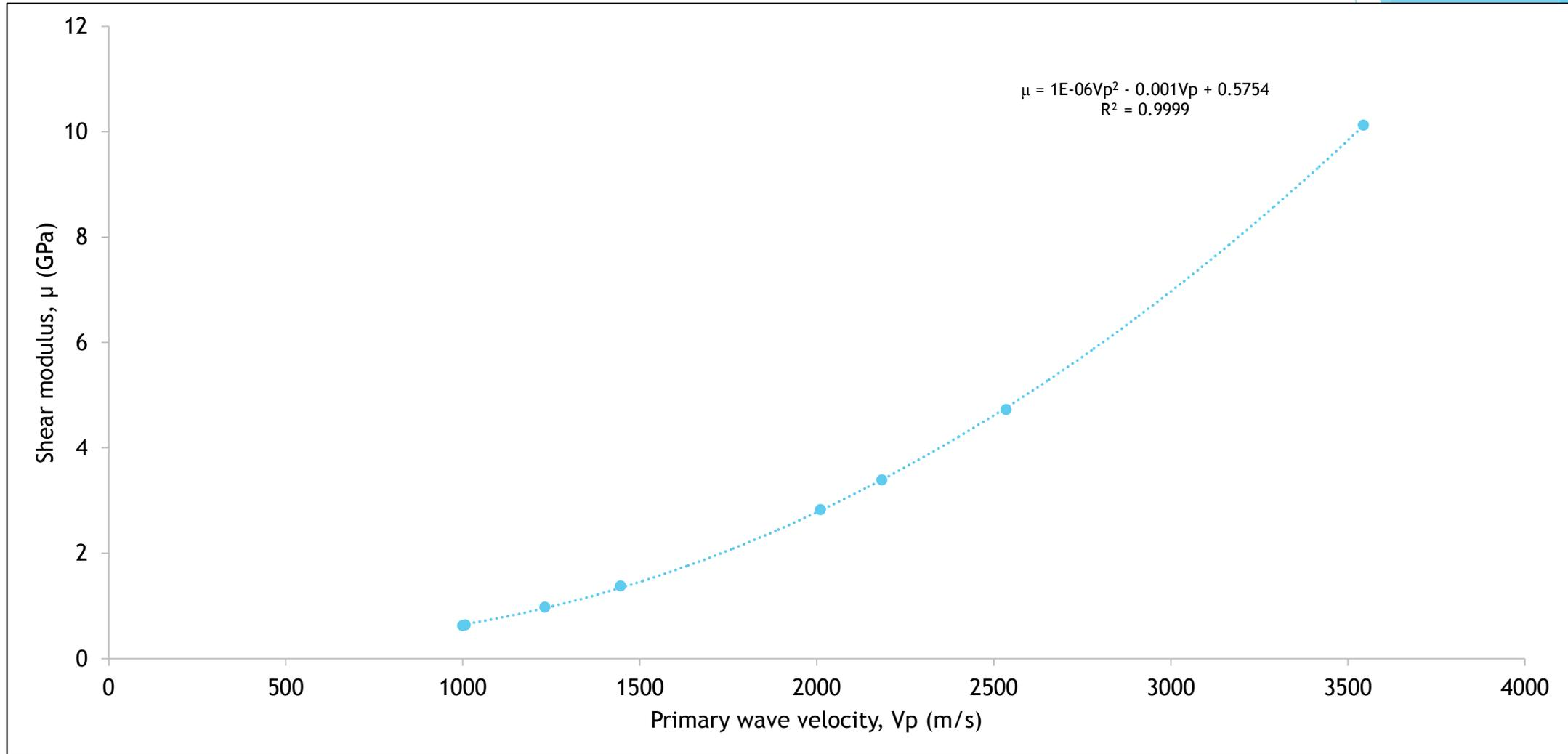
Fig 4: The graph of shear modulus (GPa) against primary wave velocity (m/s)
