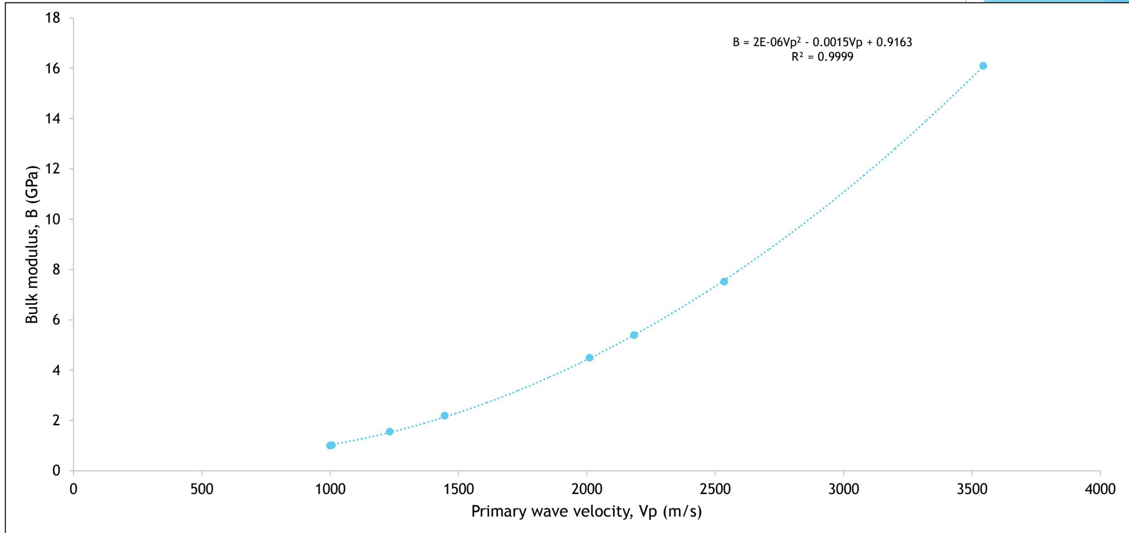
Fig 3: The graph of Bulk modulus (GPa) against the primary wave velocity (m/s)
