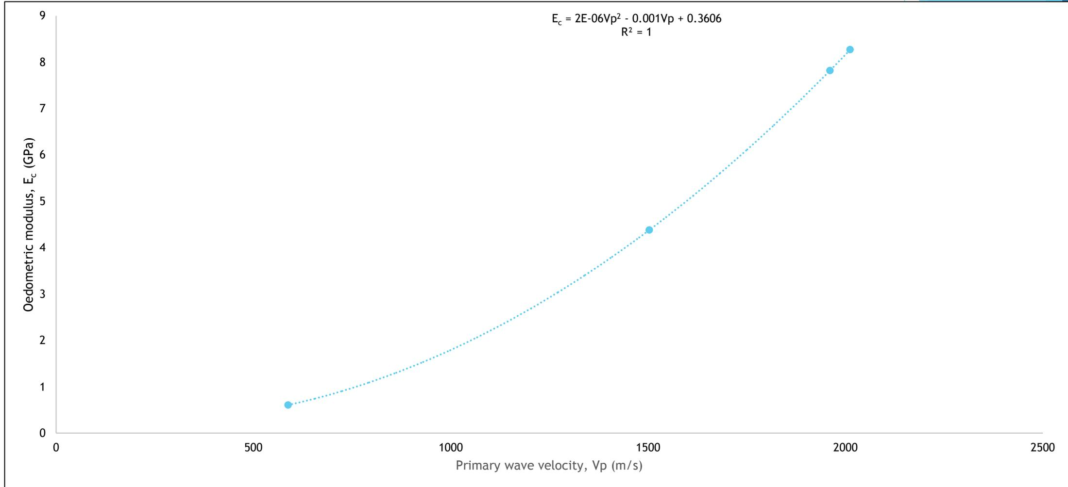
Fig 5: The graph of Oedometric modulus (GPa) against primary wave velocity (m/s)
