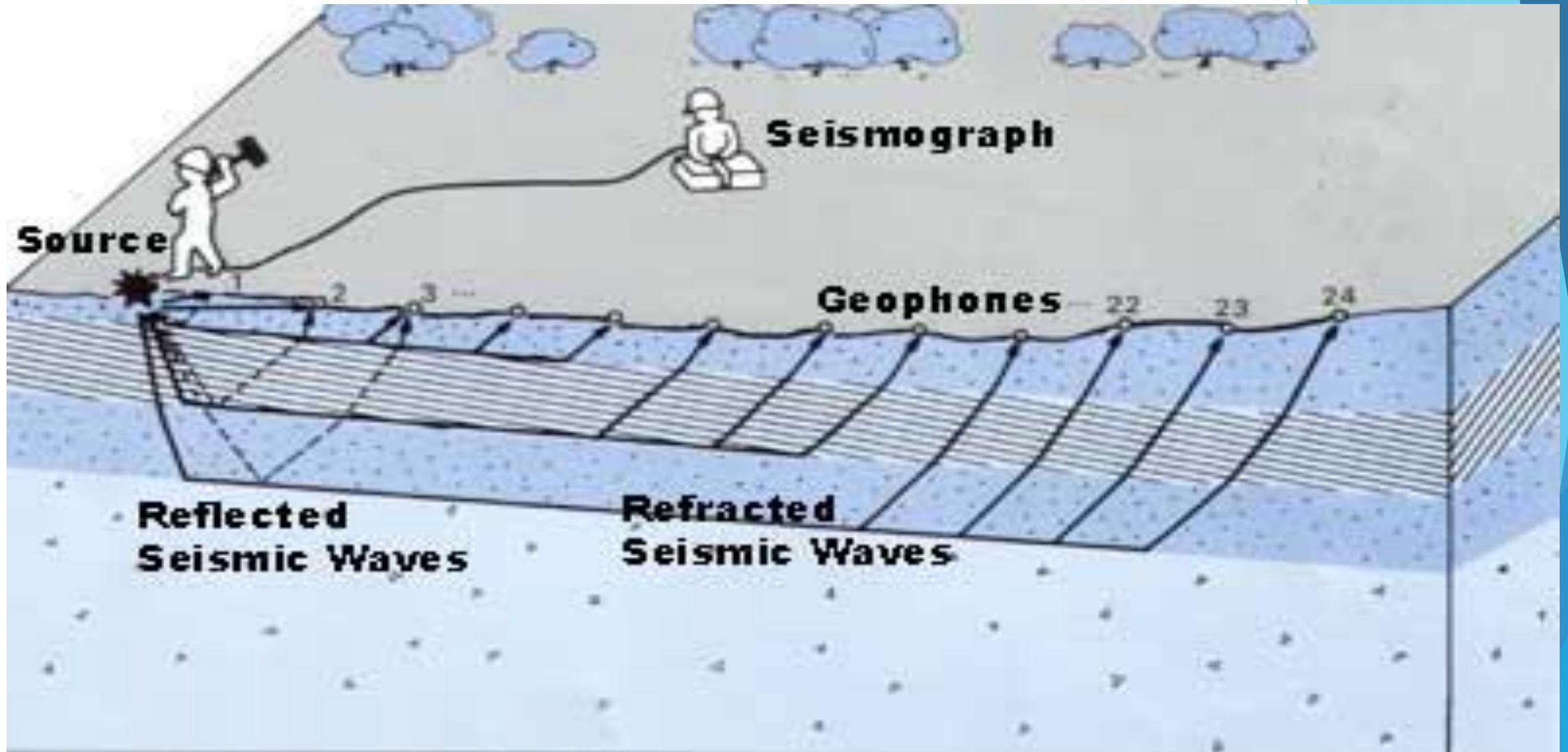
Fig 1: schematic diagram of seismic refraction method (Subsurface geotechnical, 2016).
