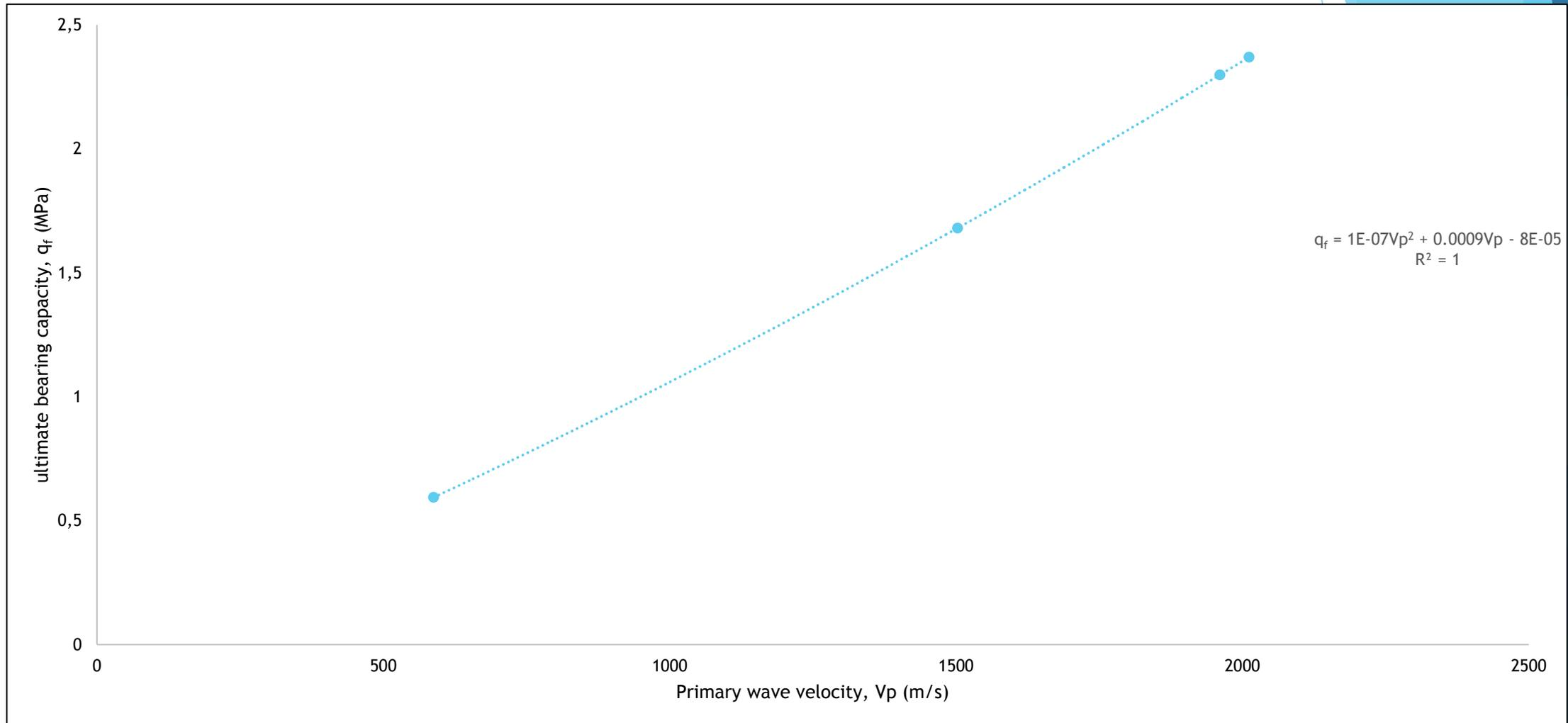
Fig 6: The graph of ultimate bearing capacity (MPa) against the primary wave velocity
