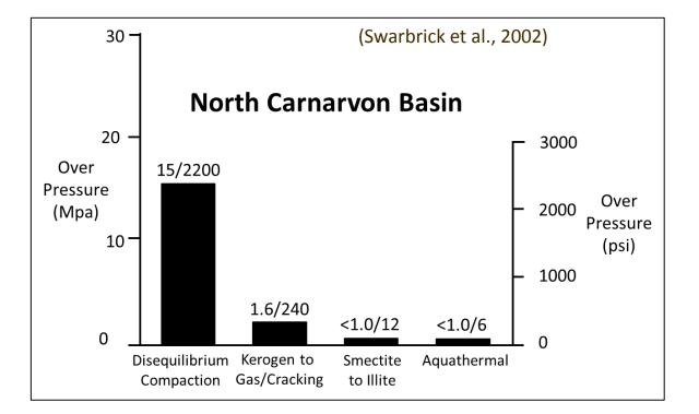
"Magnitude of overpressure from fluid expansion mechanisms is controlled by the rate of volume change which might be slow for the burial rates and temperature gradients found in most basins."
