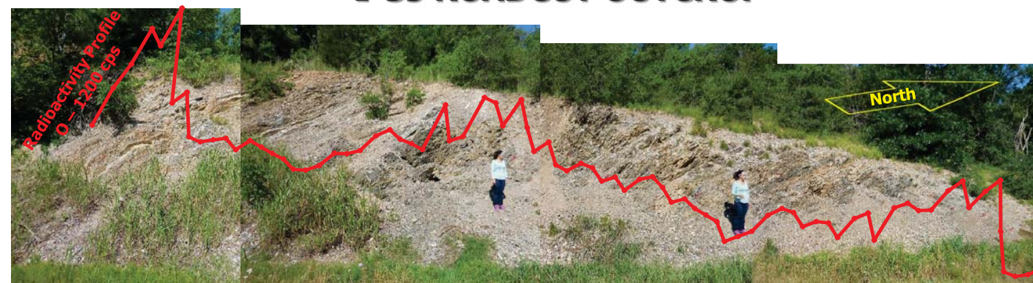
Exposure of the Woodford shale along the interstate-35. Illustrating the thin-bedded character and the radioactivity variations from base towards the top. Beds are dipping 240/45°SW. Measured stratigraphic thickness is 80 feet.
