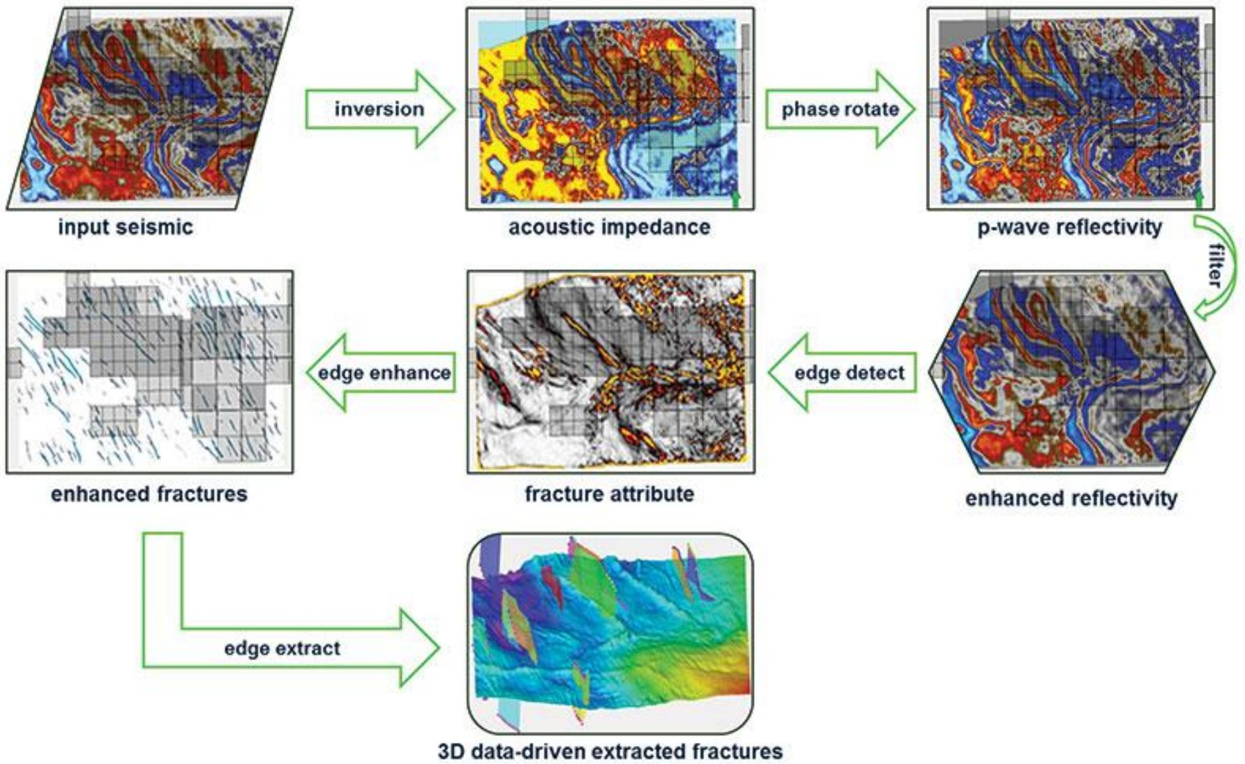
Figure 1. Seismic data-driven high-resolution fracture extraction workflow.
