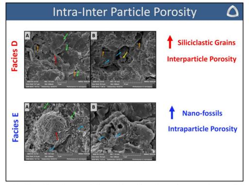
Presenter's notes: Both intraparticle and interparticle porosity was present in this reservoir. Interparticle porosity was much more common in areas near siliciclastic grains, especially in areas with larger grains as seen above. Intraparticle porosity was more prolific in areas where nano fossils were more abundant and better preserved. The bottom micrograph was one of the few cocosphers that I was able to locate in Facies E and you can see the available pore space present within it.
