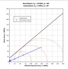
**Linear** failure criteria for rock matrix and laminations. \*Matrix contains laminations.
