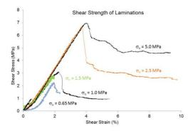
Shear strength measurement of specific laminations using direct shear testing.
