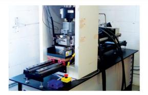
Shear strength measurement of specific laminations using direct shear testing.
