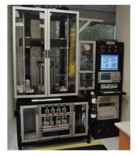
Triaxial testing of core for elastic properties and strength
