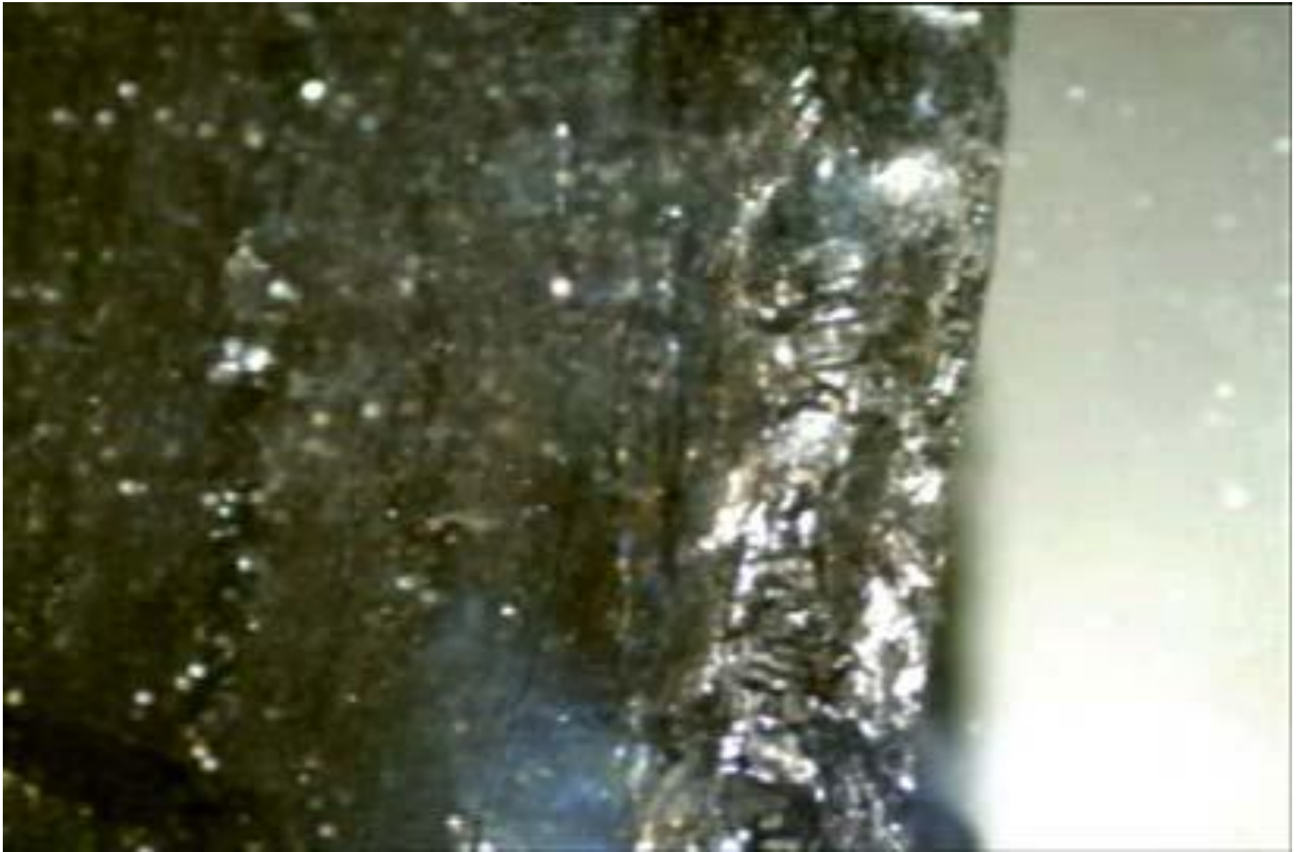
Figure 8. Representative photomicrograph of a sub-bituminous coal that is undersaturated (i.e. held in region A in Figure 7 ). Image is 7.2 mm wide.
