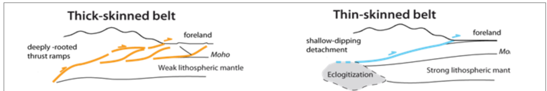
Figure 1. Main tectonic styles observed in FTBs and their relationships with continental lithosphere deformation after (Mouthereau et al., 2013).
