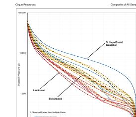
CODELL SANDSTONE Injection Pressure vs Mercury Saturation
