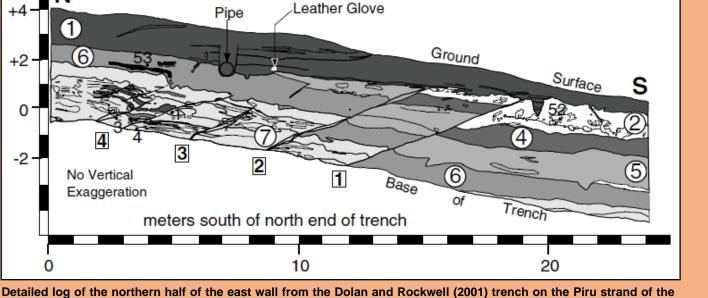
San Cayetano Fault. Numbers in square boxes denote the four principal fault strands. Small black dots show locations of detrital charcoal samples. Note strands 1 and 2 accommodated the most reverse slip during the most recent rupture event. Horizontal scale is distance, in meters, measured from the north end of the trench. Vertical scale is meters above or below an arbitrary datum near the base of the north end of the trench. (modified from Dolan and Rockwell, 2001)
