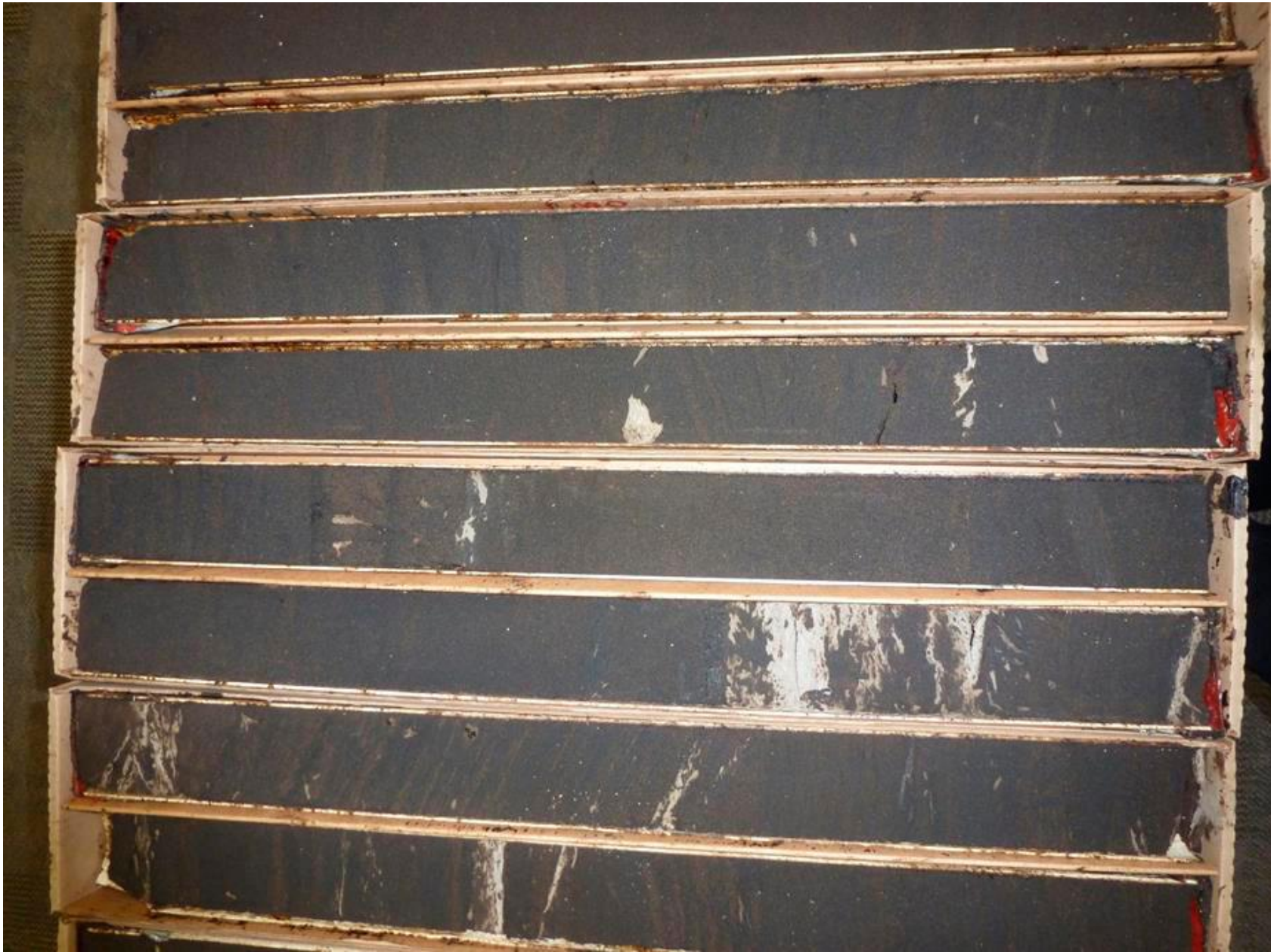
Figure 4. Ripple-cross laminated and cross-bedded sands from 1AA/09-27-094-11W4. Note the variable dipping cm-scale mudstone beds associated with fore-set beds and drapes, interpreted to have limited lateral extent based on core and outcrop data.
