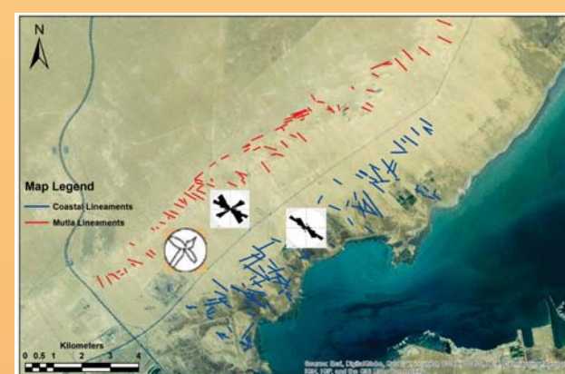
Figure 12: Comparison of Lineament Trends (squares) with Joint Trends (circle) in the Jal Az Zor Area (Basemap: Esri Webmap, 2012)
