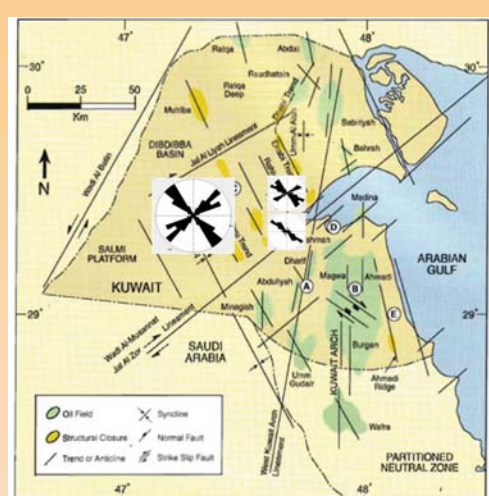
Figure 17: Comparison of Mapped Lineament Trends with Major Structural Elements of Kuwait (Carmen, 1996)
