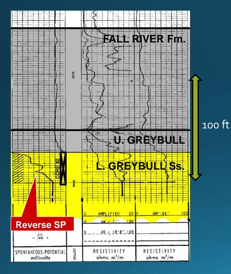
Six miles west of and more than 1100 feet downdip to the Mosser Dome oil field, this well encountered abundant heavy oil saturation in the Lower Greybull sandstone as seen in the core description below.
