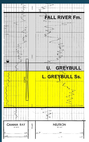
CORE: 905-990' (GREYBULL Ss.) REC 80' SANDSTONE, FINE TO MEDIUM GRAINED, SLIGHTLY CALCAREOUS, WITH LIGHT BROWN OIL STAIN IN TOP 3 FEET
