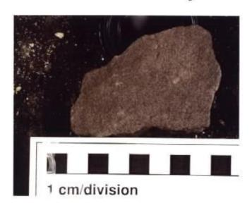
This rock sample is from outcrops on the southeast edge of the Mosser Dome stratigraphic trap. Note the abundant oil coating the quartz grains.
