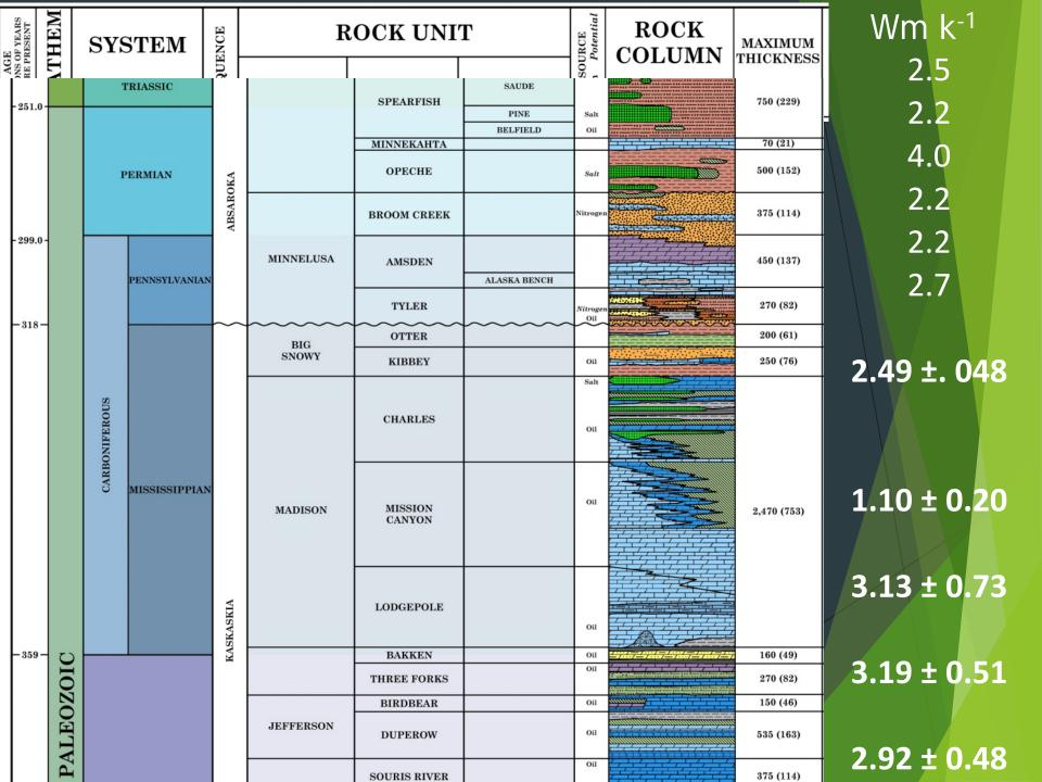
The geothermal gradient varies inversely with thermal conductivity
