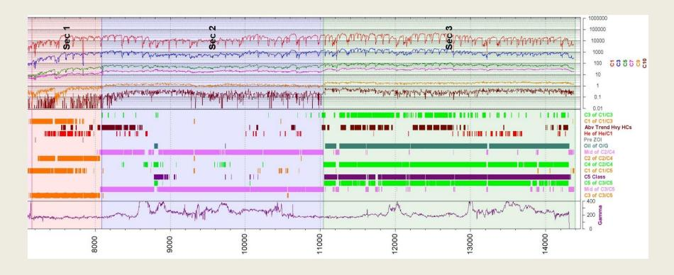
So, instead of trying to look at curve data visually we have tested a number of x-plots, chosen analytic conditions, and displayed these as "DNA". This type of analysis is not all that we do with gas data; we make smaller footage range x-plots for instance, but this is an essential part of our flow compartments analysis.
