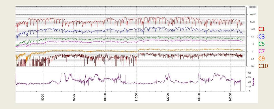
For an actual lateral shale well the mud gas readings look like this in log form. Other than speculation about apparent gas volumes this type of information is not especially easy to use. So let's look at some of this very same data another way.
