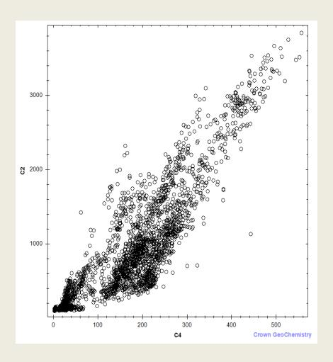
For this same lateral well every foot drilled had a reading for C2 and for C4.
