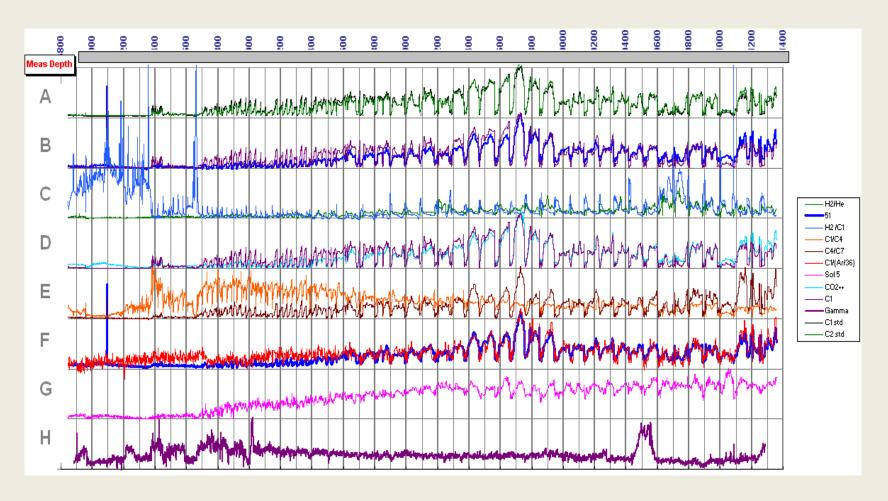
This particular well happens to have very good gas data (collected with the patented new Gas Cannibal ™ gas extractor from F.I.T. Inc.). This lateral has only mild stratigraphic variation helping isolate interpretation techniques. Certainly things may be learned using this type of linear graph in conjunction with other available analysis; for instance, the eye falls to the high apparent volumes toward the middle of and low values toward the toe of this lateral.
