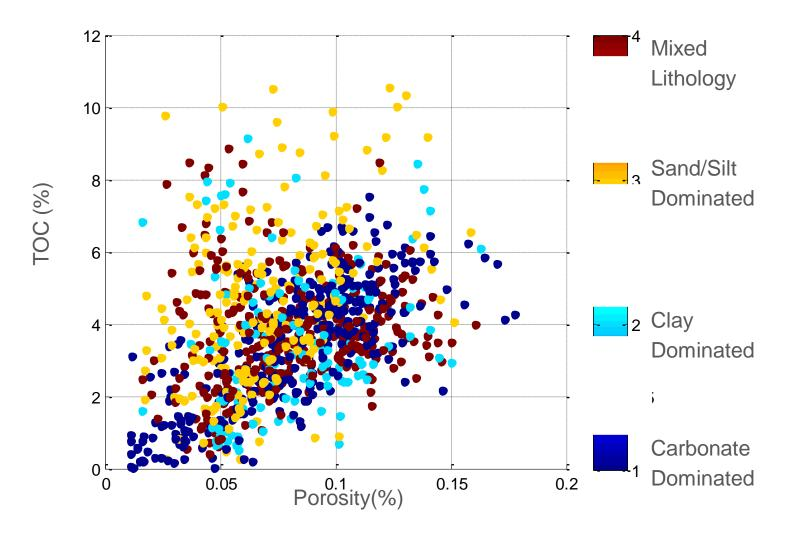
Carbonate dominated lithology shows low TOC at low Phi.
