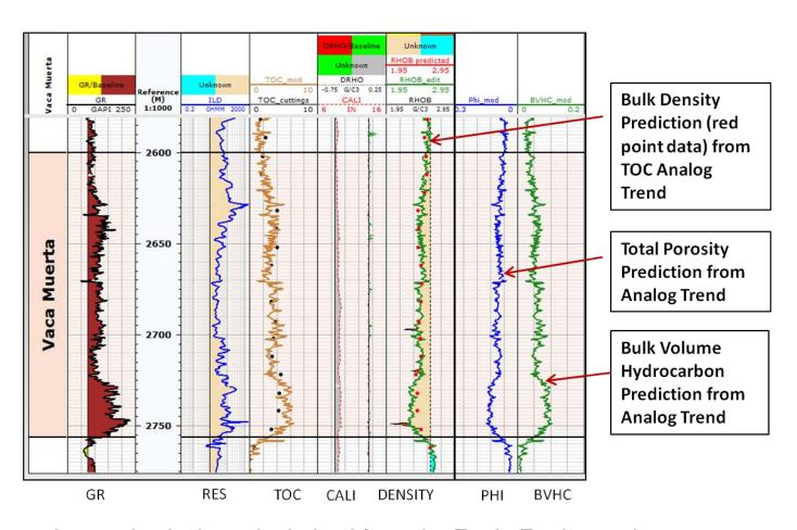
Core based petrophysical trends derived from the Eagle Ford core data were used to predict TOC, Porosity and Bulk Volume Hydrocarbons in the Vaca Muerta Well.
