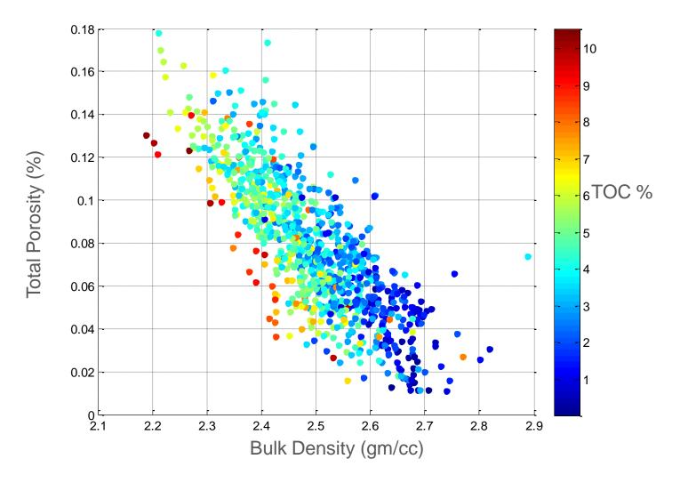
Potential to derive TOC content from Bulk Density – Porosity trend.
