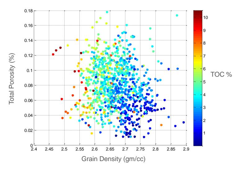
At a given Porosity, TOC content has a major effect in lowering Grain Density.
