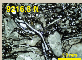
9216.8 ft: Very dark gray phosphatic wackestone rich in highly-abraded and recrystallized crinoid and other skeletal debris together with phosphate nodules.
