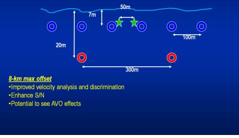
Presenter's notes: Description of main elements of the DISCover Technique: 6 cables over at 7m depth, 100m separation, 8000m offset; 2 cables under at 20m depth, 300m separation; V-frame source array, flip/flop, 50m source interval.
