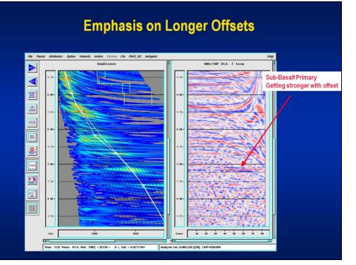
Presenter's notes: Velocity "picking" clearly emphasizes non-hyperbolic events over the longer offsets, a technique that is a <u>must</u> (long-offset data) for imaging of sub-basalt. Energy scattered--to end up on far traces.
