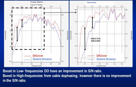
Presenter's notes: Frequency bandwidth gains produced with the DISCover technique. The combined dataset has significance in signal levels up to and in excess of 0-15Hz.
