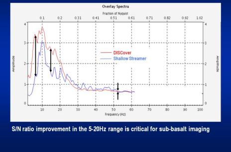
Presenter's notes: Signal/noise ratio (input to migration). The combined dataset has significance in signal levels up to and in excess of 15Hz.
