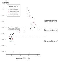
Propane carbon isotope ratios against depth showing similar isotope values despite different sampling techniques. The reverse trend beginning at ~1500m is called the isotope rollover (C2 or C3)
