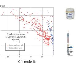
At the same depth an isojar may indicate 20% methane (red circle) whereas the equivalent isotube will indicate more than 80% methane
