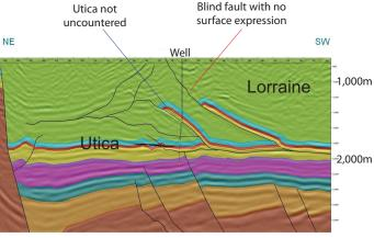
The seismic was interpreted prior to drilling the well. The faults were encountered where predicted by the seismic (depth converted). However, the Utica was not present where predicted in the hanging wall of the faults and only Lorraine was recognized.
