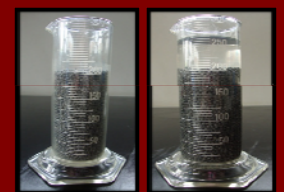
Figure 4. V_{\text{pores}} = V_{\text{sample}} + V_{\text{water}} - V_{\text{final}}
