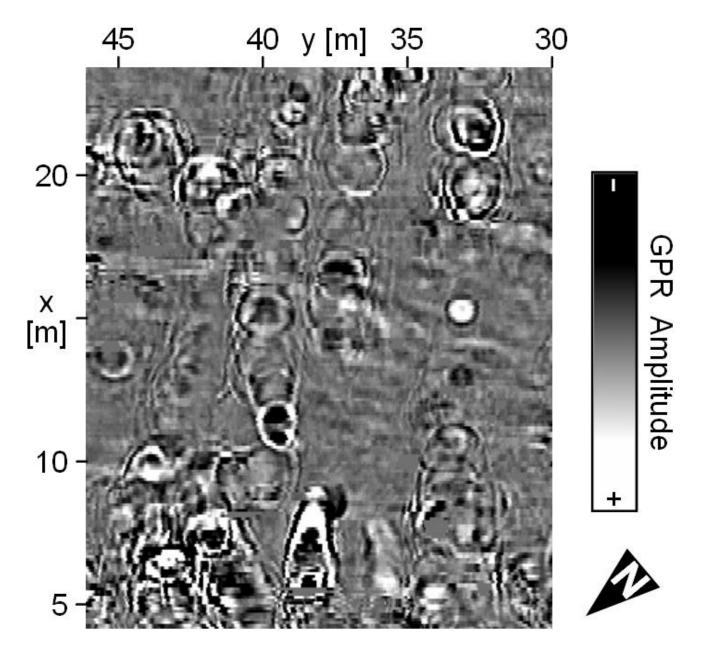
Figure 2. Unmigrated horizontal slice extracted at 1.95 m depth with abundant diffractions.
